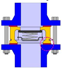
Larger flange facings prevent "flowing" of the asbestos-free flange gaskets and jamming of gaskets during installation.
